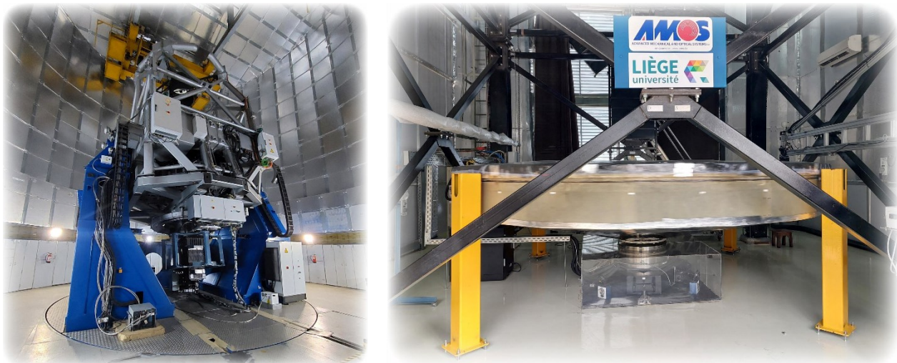
Figure 5: The 3.6-m Devasthal Optical Telescope (left) has a conventional glass mirror while the 4-m International Liquid Mirror Telescope (right) is a zenithal telescope having a mirror consisting of a thin layer of liquid mercury.
